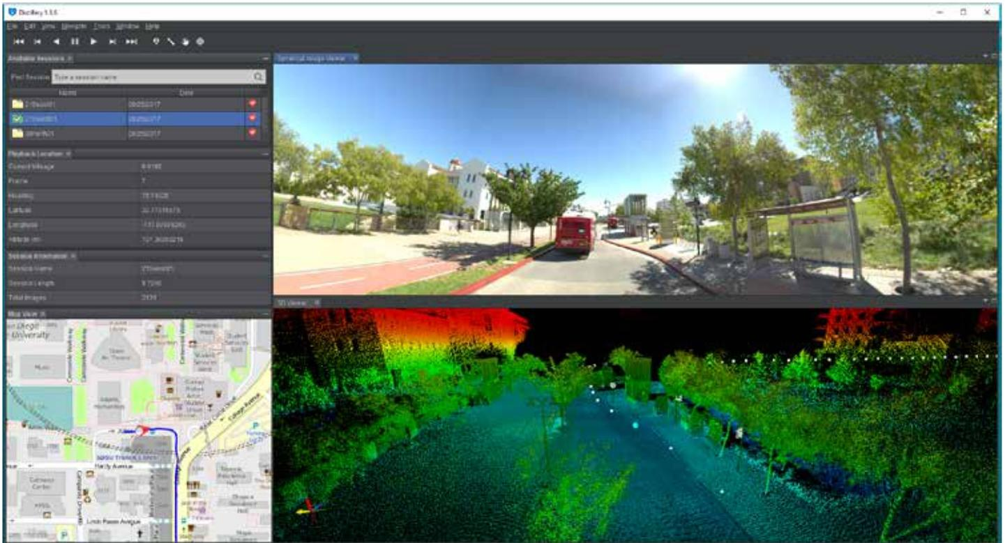
» The point cloud, 360 degree imaging, and map view are shown within Maverick's post-processing software, Distillery. Several assets of interest are identified within the dataset, including the bus stop, shelter, bench, and garbage cans.
