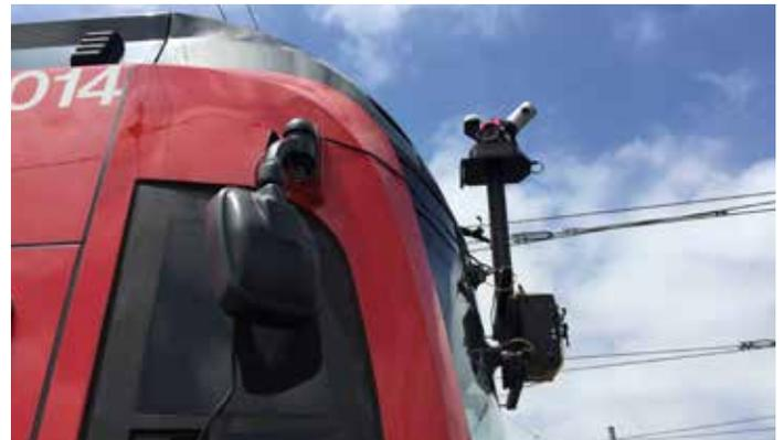
» Maverick mounted to a commuter train with Mandli's prototype suction cup mount. The mount is powered by a vacuum pump with an internal backup battery housed within the control box.
